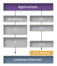
Figure 3 Networking and Fibre Channel stacks
